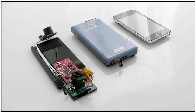
Figure 2. The components used in our prototype. From left to right, a sensor unit, a handheld projector, an iPod Touch.
