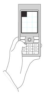
**Figure 3.** The *TwelvePixels* interface, keys are spatially mapped to pixels on screen.
