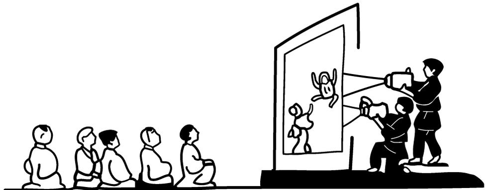
light passes through the slide and on through the projection lens to enlarge the slide image.
